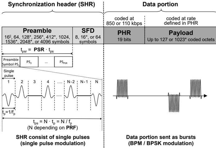
Fig. 1. UWB PHY frame structure according to the IEEE 802.15.4 standard. Settings marked with \* are also available in the Decawave DW1000 transceiver, whilst the ones marked with || are not supported [23].
