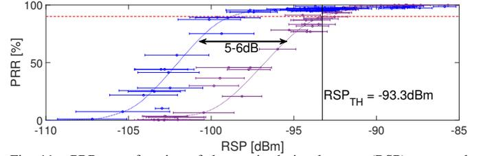
Fig. 11. PRR as a function of the received signal power (RSP) measured using the DW1000 default settings (violet) and a data rate of 110 kbps (blue).
