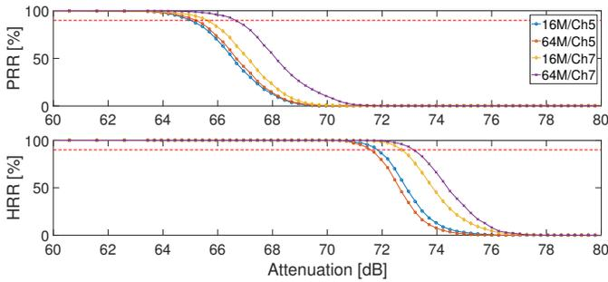
Fig. 6. Packet reception rate (PRR) and header reception rate (HRR) for different attenuation levels as a function of pulse repetition frequency (PRF).
