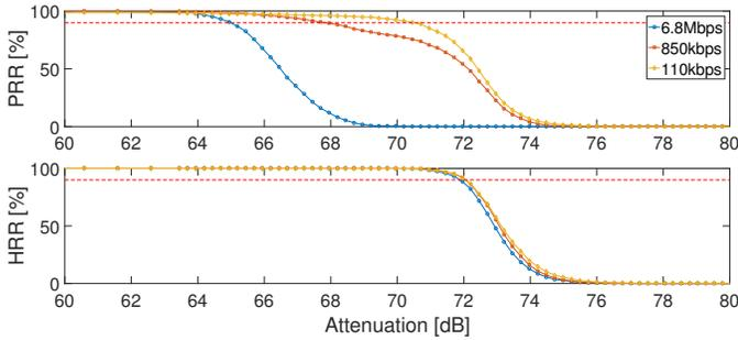
Fig. 7. Packet reception rate (PRR) and header reception rate (HRR) for different attenuation levels as a function of data rate.
