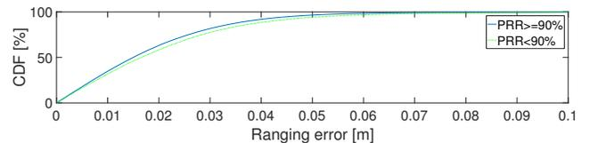
Fig. 9. Cumulative distribution function (CDF) of the ranging error. Solid blue line for reliable links and green dotted line for unreliable links.
