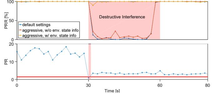
Fig. 14. The proposed adaptation scheme can correctly recognize and escape destructive interference, sustaining a high reception rate over time.
