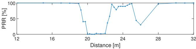
Fig. 3. Decrease in packet reception rate (PRR) caused by destructive interference in a multipath-rich indoor environment.
