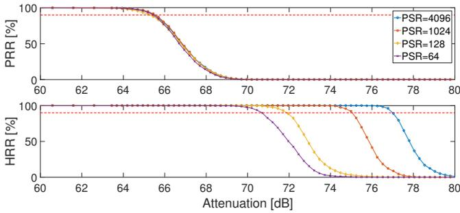
Fig. 5. Packet reception rate (PRR) and header reception rate (HRR) for different attenuation levels as a function of preamble symbol repetitions (PSR).
