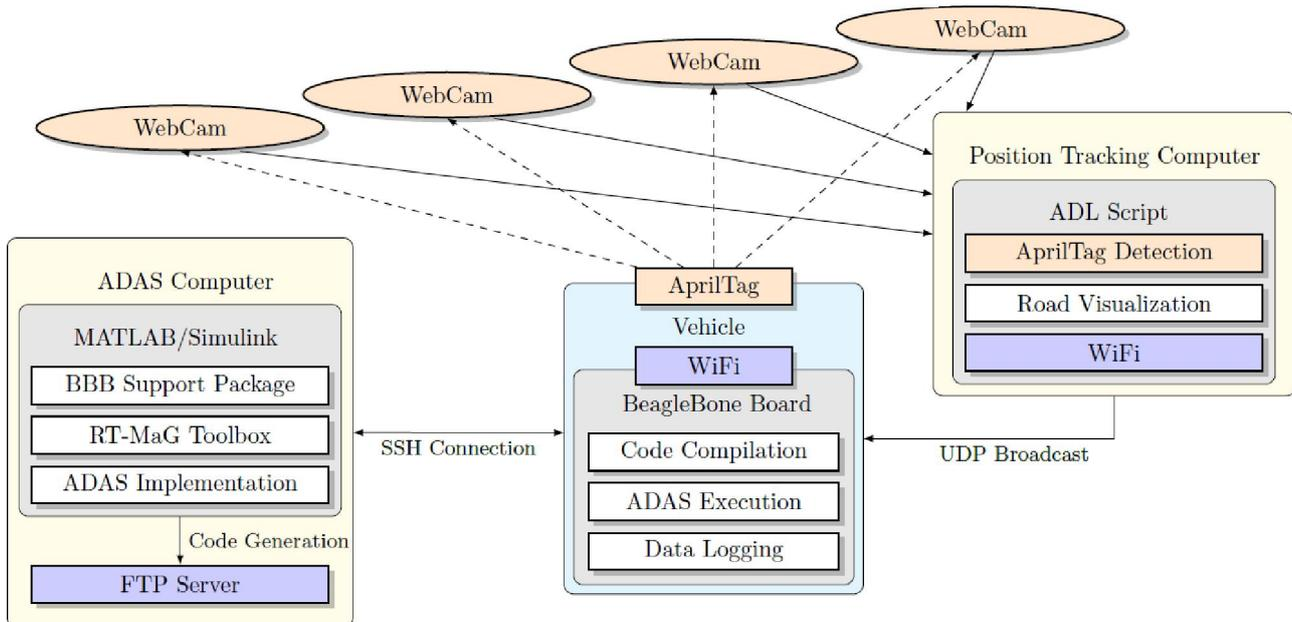
Fig. 13 – Setup of the testbed using small-scale vehicles and communication.
