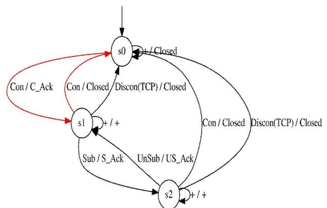
Fig. 6 – FSM model of the Mosquitto MQTT broker.
