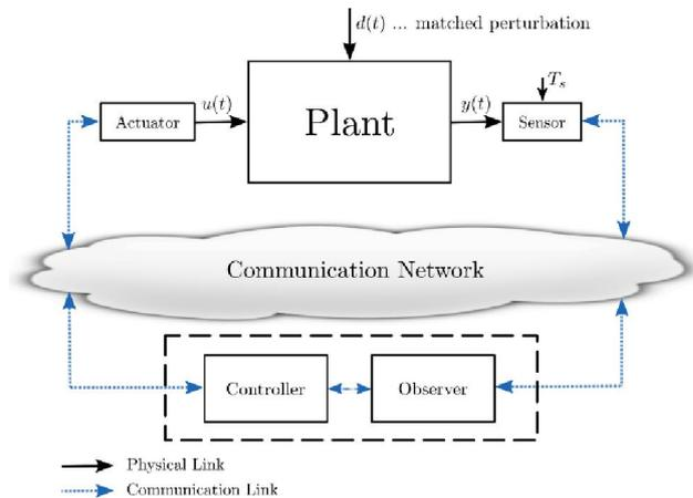
Fig. 9 – Structure of a Networked Control System.
