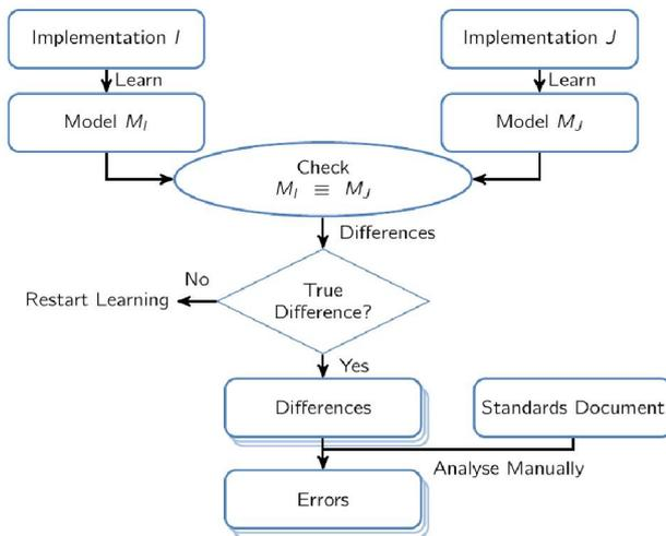
Fig. 7 – Overview of learning-based protocol testing.
