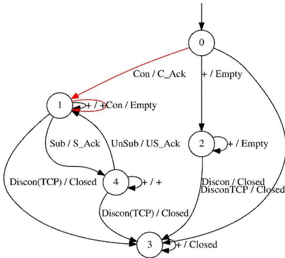
Fig. 8 – FSM model of the HMQTT broker.
